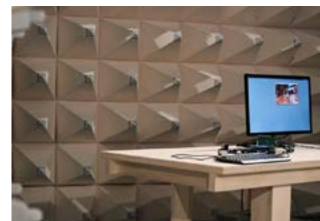
Figure 38: Arezzo plant, interior view of the anechoic chamber
